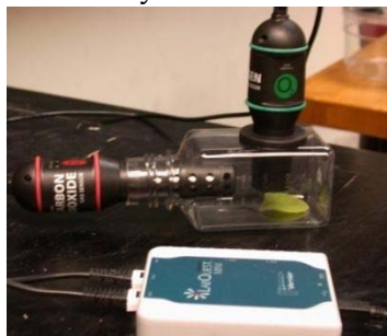
Respiration chamber, sensors and hub.
