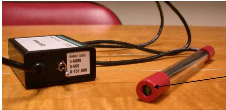
The light sensor is located here and the light must hit this surface.
